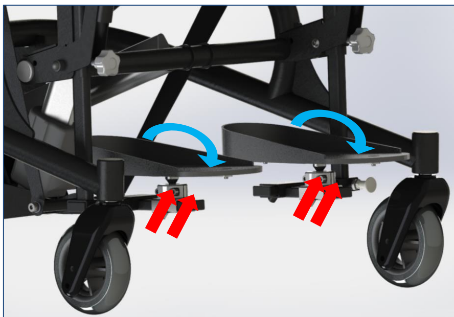
* Fig 17: The adjustment angle of feet platforms
