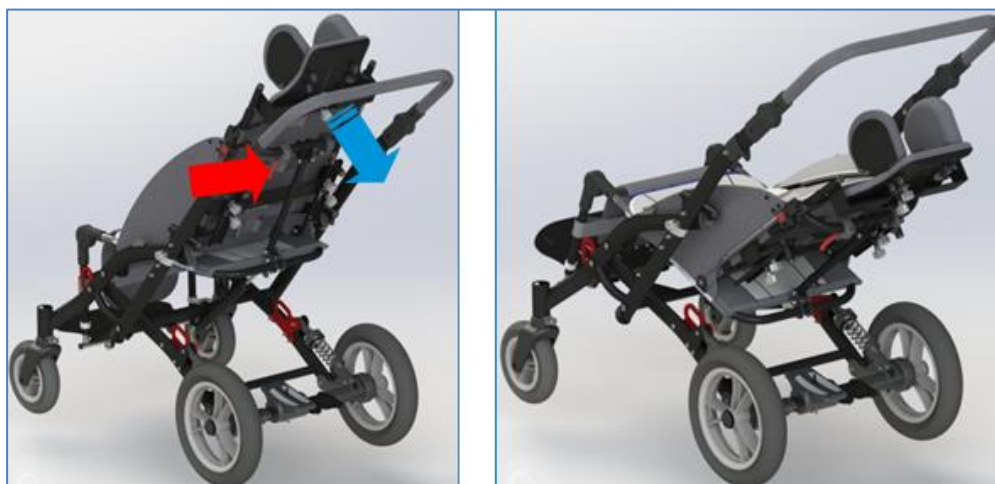
Fig. 30 Seat angle adjustment
