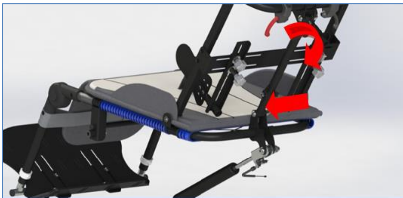
Fig. 34 Chest support width and height adjustment
