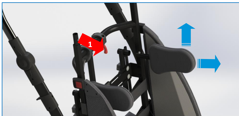
Fig. 19 Chest supports dismantling
