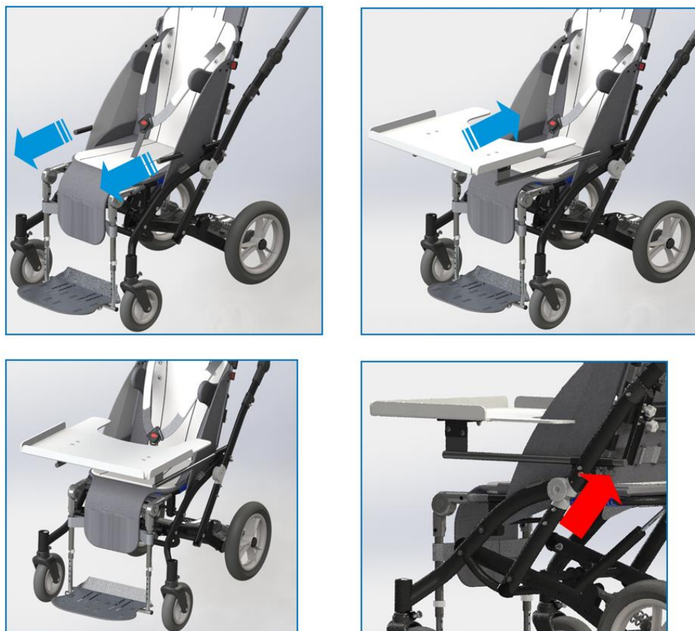
Fig. 13 Table installation
