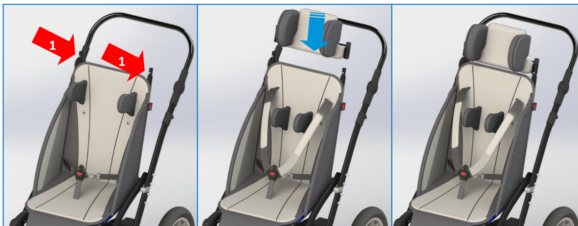
Fig. 8 Mounting the head supports
