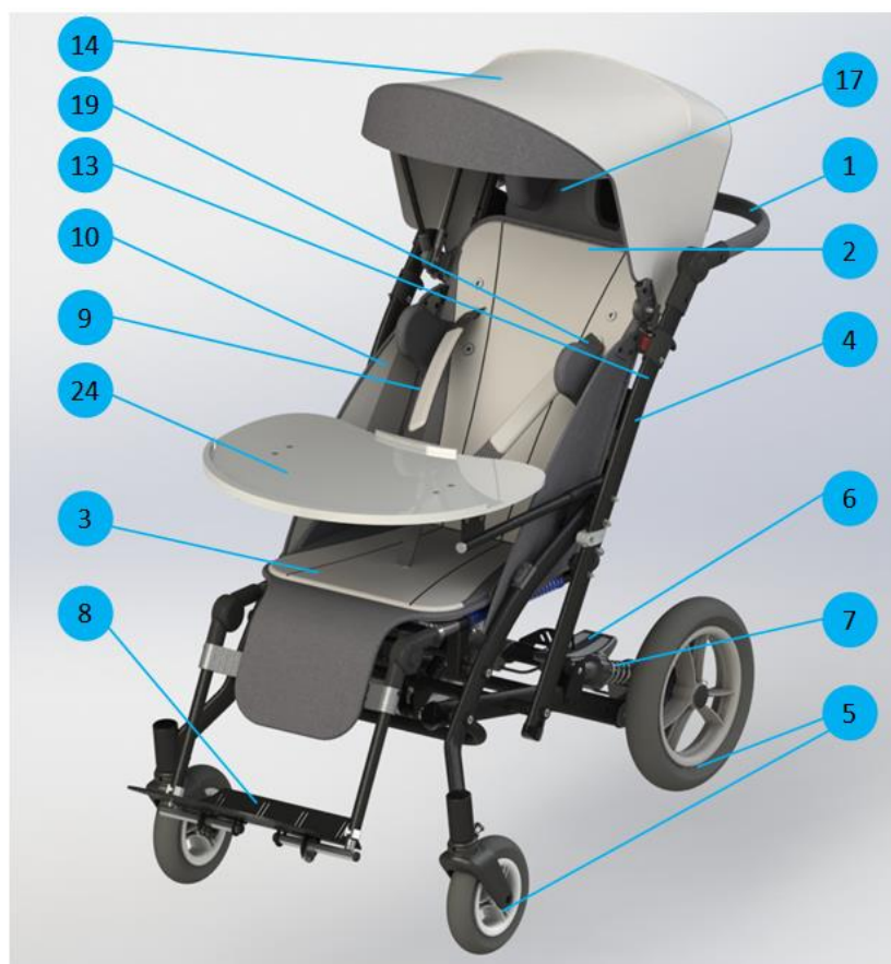
Fig. 1 Structure of the stroller
